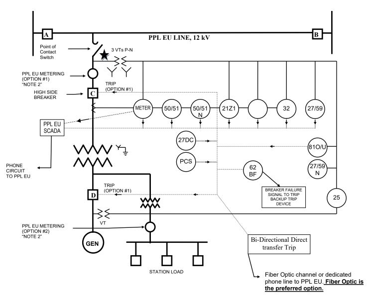
Fuses must be installed on customer VTs on the PPL side of the POC CB.
