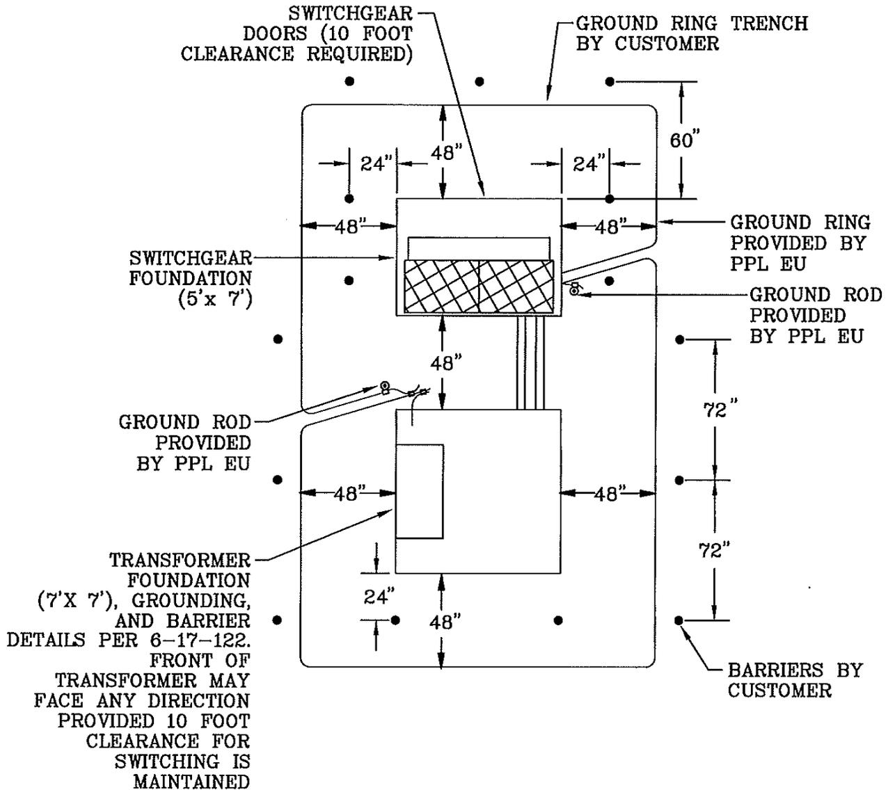
NOTE: TRANSFORMER FOUNDATION IS SET 4 INCHES DEEPER THAN SWITCHGEAR FOUNDATION
