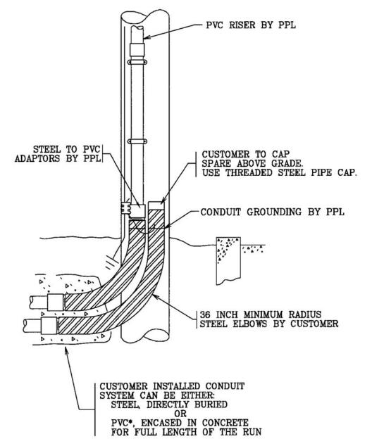
\*TO PREVENT PVC TO STEEL COUPLING FROM BREAKING, ENCASE LOWER 1/3 OF STEEL ELBOWS IN CONCRETE 6-18-115-B
